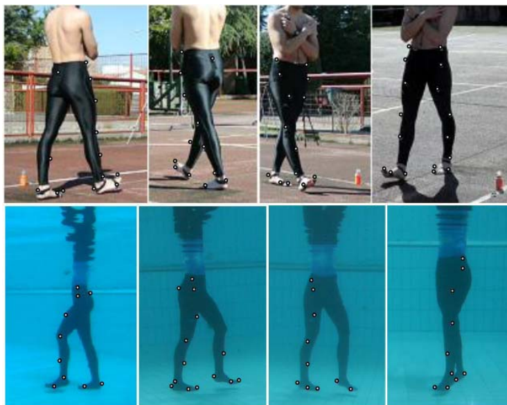
Figure 1 Four camera views during forward walking on land and backward walking in water, with marker positions indicated where visible to the camera
