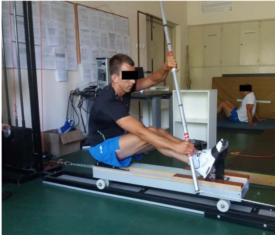
Figure 1 Single kayak stroke test performed on a custom-made machine.
